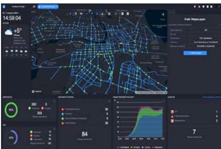
Online traffic management and adaptive traffic light control RITM 3
