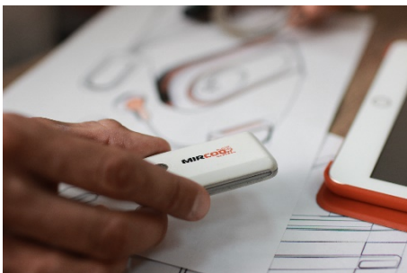
A small ECG Patch that functionally replaces bulky Holter monitoring devices.
